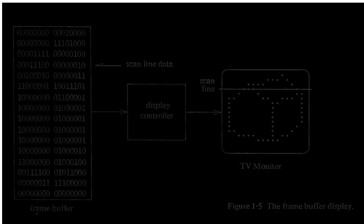
The display controller simply reads each successive byte of data from the frame buffer and converts its Os and Is into the corresponding video signal. This signal is then fed to the TV monitor, producing a black-and-white pattern on the screen, like the wheel shown in Figure 1-6. The display controller repeats this operation 30 times a second and thus maintains a steady picture on the TV screen.
